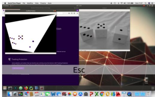
Figure 4: Visual recognition system of the die numbered faces on a surface.
